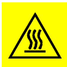
High Temperature Alarm Label
